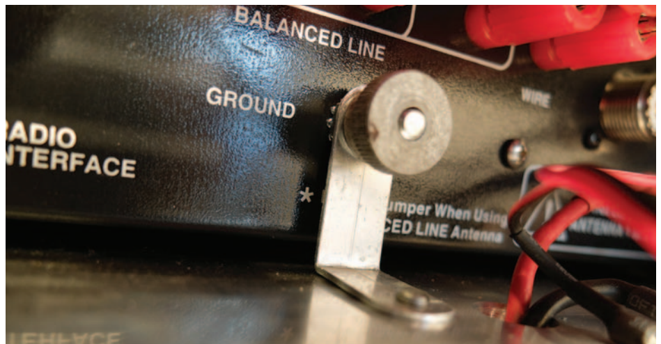
PHOTO 1: Earth terminal at rear of MFJ Intellituner.
