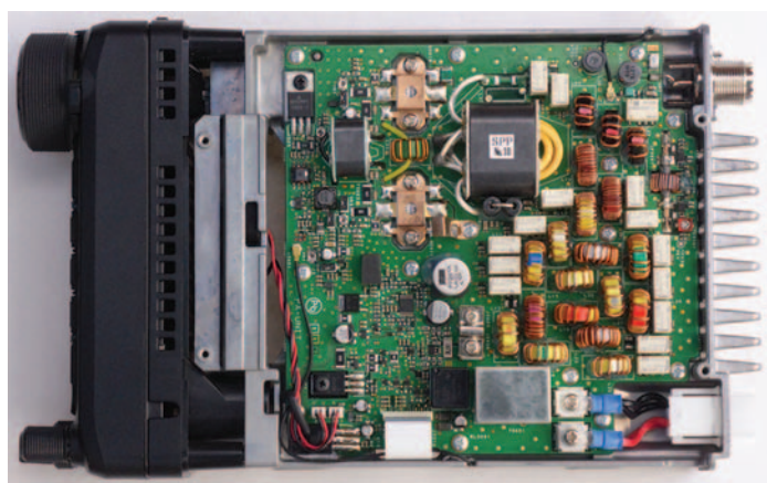
FT-891 Under the bottom cover showing power amplifier and filters.
