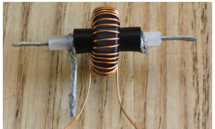
PHOTO 2: Practical configuration of a non-directional coupler.
