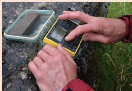
The Cave-Link system provides text-based communication between a cave and the surface.
